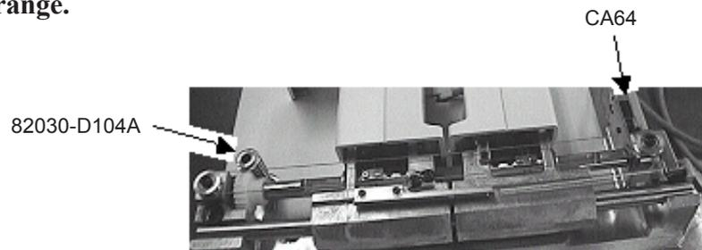
5. Adjust the position of the micro switch (CA64) so that the switch is turned on at the position where the worm gear is stopped.
